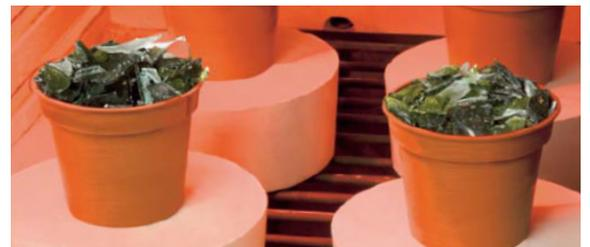
Glass in Ceramic Feeder on Mould
