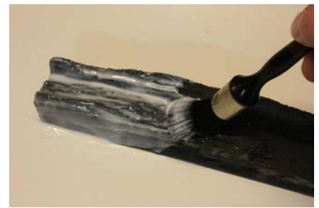
Fig. 2 : First apply a film layer of silicone on to the model. Enabling any air bubbles to get out through the film layer.
