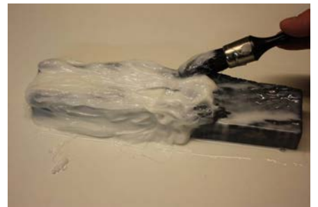
Fig. 4 : The second layer is applied. This layer will give the mould strength.
