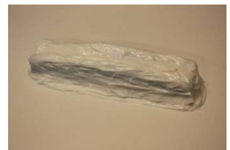
Fig. 5 : The brick slip is completely covered in a layer of +/- 5 mm silicone.
