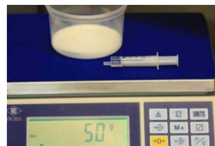
Fig. 3: The B component has a small dosage. A syringe to measure and dispense is swift and accurate. In this case you can read 1 ml as 1 mg.
