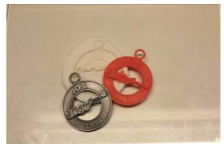
Fig. 5: The mother model, mould and a copy out of red casting wax.
