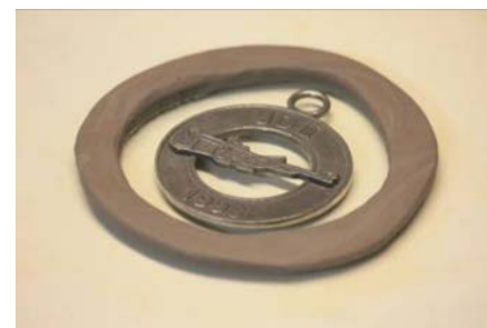
Fig. 2: Make a border of plasticine around the model as a barrier for the silicone.
