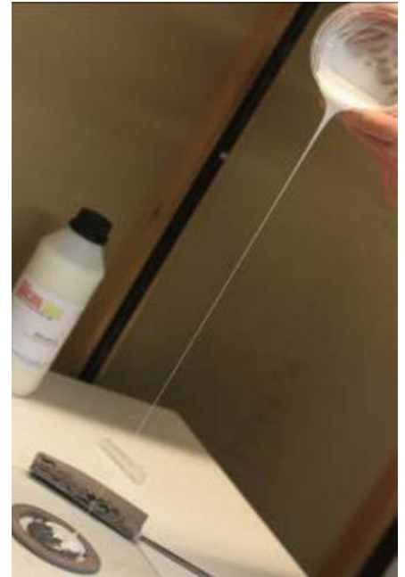
Fig. 4: Casting the silicone in a thin trickle will give air that is trapped inside the silicone time to escape.
