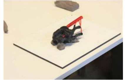
Fig. 2: The master model is set in position and wax extruders are attached
