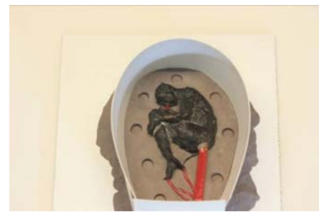
Fig. 5: The embedded model with wax extruders and formwork. Ready for silicone casting.
