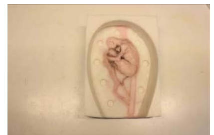
Fig. 12: After demoulding the mould will flip back any parts were cuts were made. These cuts will not show up on the copy
