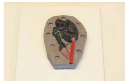
Fig. 4: Arround the model a series of indentations are made to form the key.
