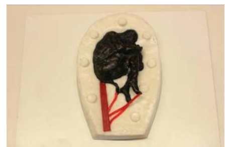
Fig. 7: The model is embedded in silicone upto the division seam. And treated with vaseline.
