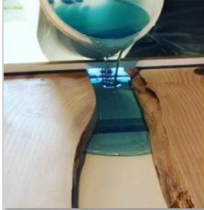
When pouring in multiple stages the best process is to allow the previous layer to cure to a firm but still tacky state, then pour the next layer on top of the partially cured layer.
