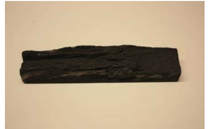
Fig. 1 : This ornamental brick slip has been cleaned unwanted dents are filled up and the surface has been treated with a release agent (vaseline).
