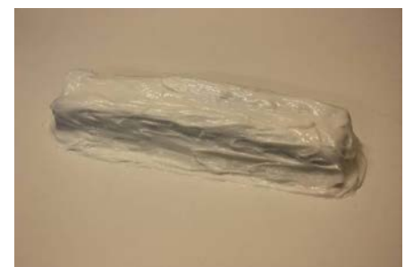
Fig. 5 : The brick slip is completely covered in a layer of +/- 5 mm silicone.
