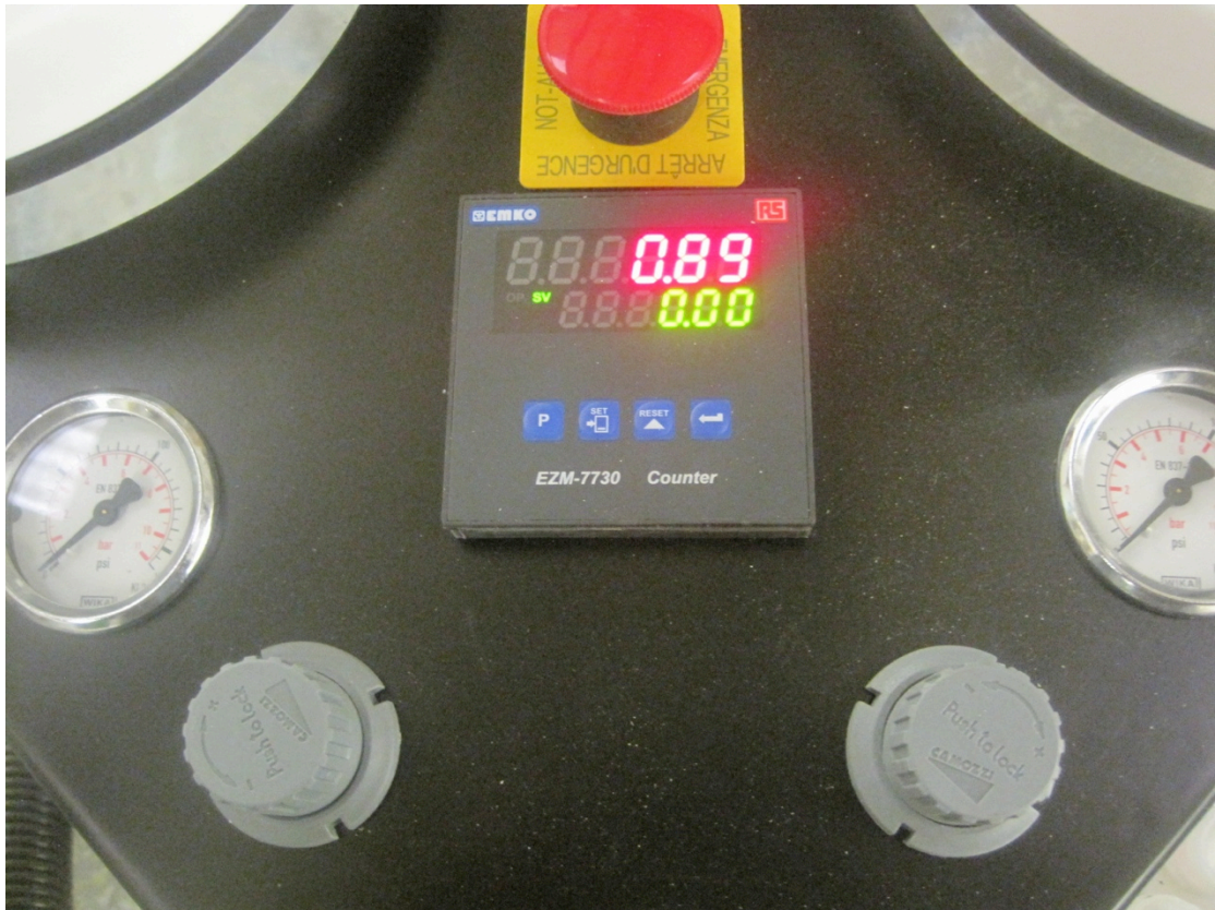
Optional Digital counter fitted . Power supply 24 VAC plugs into rear of instrument panel
